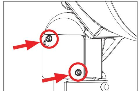
4. Fit fixture over pole on mounting plate and ensure it is completely seated. Secure fixture to pole by tightening two (2) 3/8"x16 stainless steel square screws using an adjustable crescent wrench.
