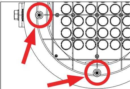
7. To relamp: remove faceplate and louver by loosening four (4) tamper resistant screws using a TORX T27 socket (1/4" bit). Relamp as needed, then reverse install.
