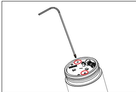
5. Use a 5/64" allen wrench to remove two (2) #2-56 socket head cap screws on LED board, grasp LED board and gently pull up to expose quick disconnect.
