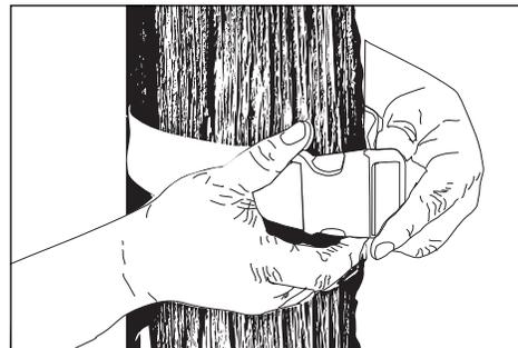
3. Use adjustable strap provided to attach UPM housing to tree. Tighten by pulling on the adjustable strap until secure.
