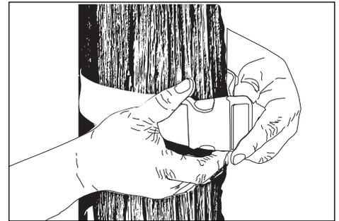
3. Use adjustable strap provided to attach UPM housing to tree. Tighten by pulling on the adjustable strap until secure.
