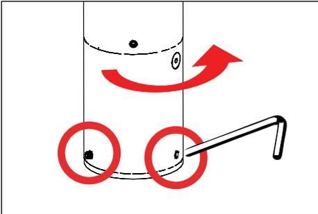
1. Use a 5/64" allen wrench to loosen (3) #8-32 stainless steel set screws on fixture base. Rotate fixture at base and aim fixture to desired horizontal location.
