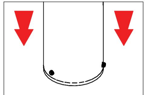
6. Place fixture onto mounted anchor base and press straight down until the two pieces are flush with each other.
