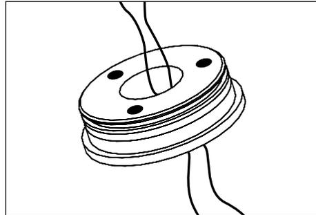
3. Pull wires from remote driver necessary for installation. Feed wiring through anchor base.
