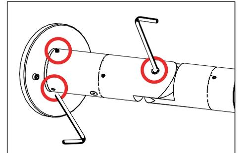
3. Tighten the three (3) #8-32 screws on base with appropriate tool for mounting method and stainless steel locking screw at the knuckle to secure all aiming positions.
