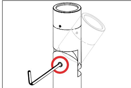
2. Use a 3/16" allen wrench to slightly loosen 1/4"-28 stainless steel black oxide socket head cap screw at the knuckle for vertical aiming purposes.
