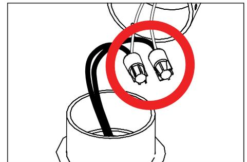
6. Make watertight connections from remote driver to fixture leads using waterproof wire connectors. **See wiring diagram.**
