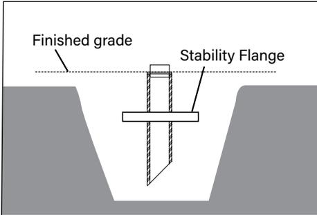
1. Excavate trench according to designed lighting plan. Dig hole a minimum of 18" deep and 10" wide to accommodate power pipe at desired fixture location(s).
