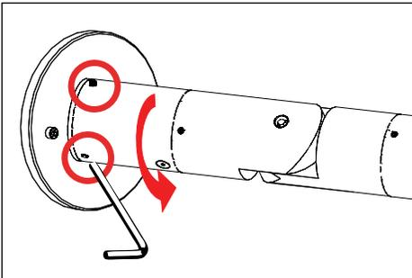
1. Use a 5/64" allen wrench to loosen three (3) #8-32 stainless steel set screws on fixture base. Rotate fixture at base and aim fixture to desired horizontal location.
