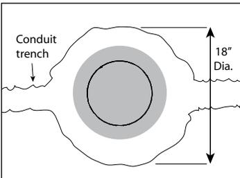
B. Excavate a hole to the necessary dimensions for fixture placement and conduit runs.
