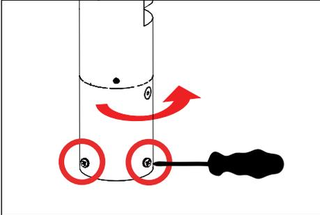
1. Use phillips screwdriver to loosen three (3) #8-32 stainless steel round head phillips screws at base. Rotate fixture at base and aim fixture to desired horizontal location.
