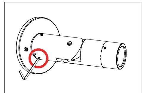
3. Use a 1/8" allen wrench to mount fixture with two (2) #10-24 hex screws to installed back box. Do not over tighten.
