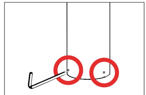
8. Tighten three (3) #8-32 stainless steel round head Phillips screws at base and 1/4"-28 stainless steel black oxide socket head screw at the knuckle to secure all aiming positions.
