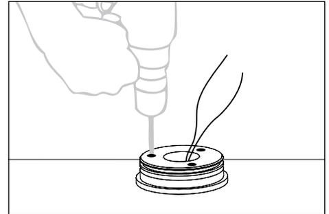
4. Secure anchor base to solid surface (i.e. wood, concrete) using appropriate hardware for specific surface.
