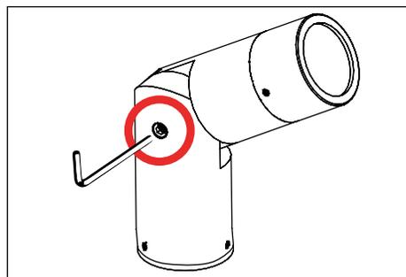
8. Tighten the three (3) #8-32 stainless steel set screws on anchor base and 1/4"-28 stainless steel locking screw at the knuckle to secure all aiming positions.
