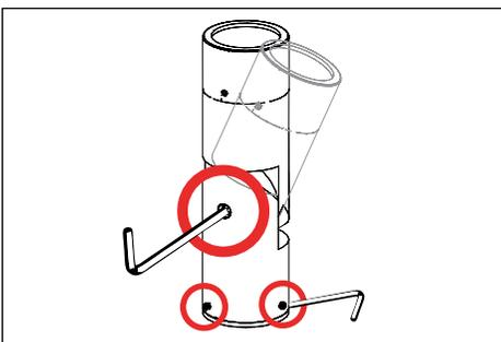
7. Use a 3/16" allen wrench to slightly loosen 1/4"-28 stainless steel black oxide socket head cap screw at the knuckle for vertical aiming purposes. Rotate fixture at base and aim fixture to desired horizontal location.
