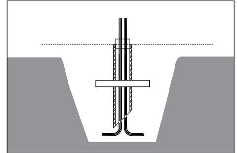
3. Pull wires from remote driver necessary for installation through power pipe. Allow for additional cable to make connections to fixture lead and future service. Place power pipe in hole.
