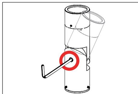
7. Insert wires and connectors into fixture base and attach to power pipe. To aim fixture, use a 3/16" allen wrench to slightly loosen 1/4"-28 stainless steel black oxide socket head screw at the knuckle for vertical aiming purposes. Rotate fixture to aim to desired horizontal location.
